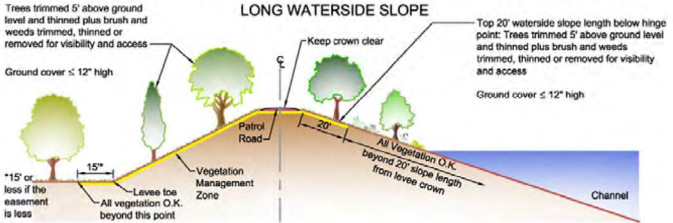
Figure F-1: Vegetation Management for Existing Levees with a Long Waterside Slope
